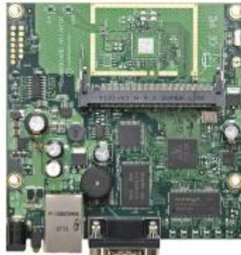
The heart of RB411 is the new Atheros CPU which makes this tiny device a quick one. Tests show that it is up to three times more powerful than our previous model.
